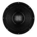
This next evolution subwoofer uses a new, longer, four layer aluminum voice coil. The result is more energy in the gap, less heat, higher sensitivity, higher power handling, lower distortion and better overall performance. The 15DS115 features a 40mm long, 4.5 inch diameter (116mm) Copper Clad Aluminum Wire voice coil. With a 1600watt AES power rating, 97 dB sensitivity, and over 14 mm of Xvar, this high energy subwoofer is a significant step forward from similar models in the B&C range.
